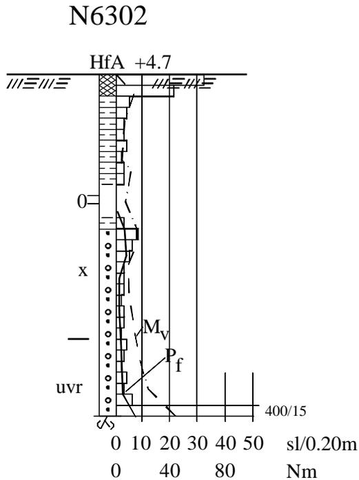
Is carried out according to method A or B. The penetration resistance is noted as the number of blows required per 0.2 m of penetration (sl/0.2 m) and is presented in a bar chart. Different scales can be used. The turning resistance ( $M_v$  in Nm) and calculated frictional resistance ( $P_f$  in sl/0.2 m) can be left out. Estimated soil types in connection with the sounding operation can be noted in the borehole column.
