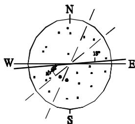
Presentation of fractures in a so-called stereo net (Schmidt diagram). The plan of the fracture is shown with a point, the pole of which is a projection of the point where a normal to the plan intersects the lower hemisphere. The observations can be brought together to form interpreted main directions represented by the broken lines in the fracture diagram.
