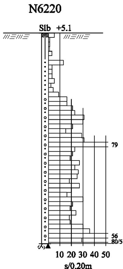
The resistance is shown as penetration time per depth interval (sec./0.2 m) and is presented in a bar chart.
