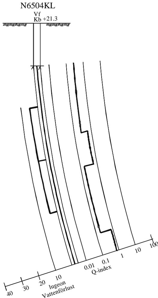
Results of core drilling can be presented in a simple or detailed way. In simple presentation in section drawings, the situation of the borehole is shown together with the values of RQD, Vf and Q/RMR. The borehole column can be utilised to illustrate the rock type. In detailed presentation there is a possibility to describe every observation made along the rock core, and for orientated core the strike and dip of individual fractures can be noted.
