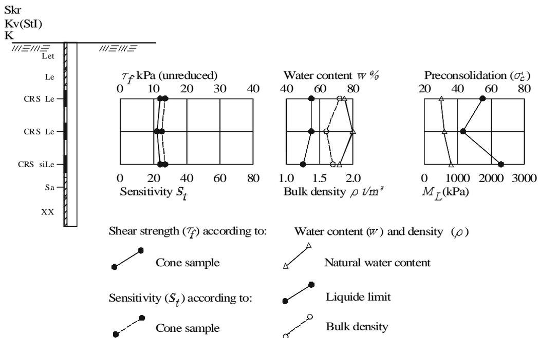
In the diagrams are presented uncorrected shear strength ( $t_k$ ) and sensitivity ( $S_{tk}$ ), water contents (natural  $w_N$ , liquid limit  $w_L$ ) and bulk density ( $r$ ), preconsolidation pressure ( $s'_c$ ) and compression modulus  $M_L$ , determined by means of oedometer tests, in this case CRS tests.
